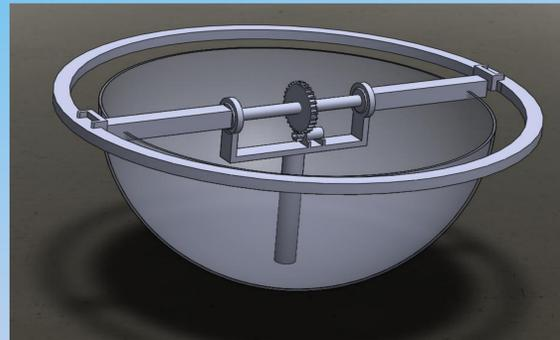
The latest model of the system. Each component is being built in small sections to be 3D printed for testing and calibration. Here you can see a motor that rotates the photovoltaic rod around the center axis. The outer circle will also rotate although this is not shown here
